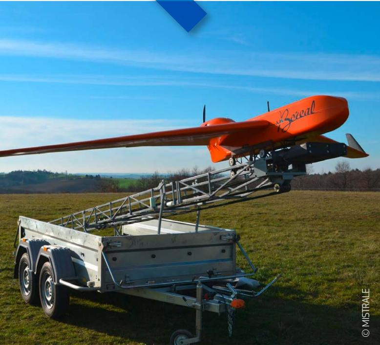
*The MISTRAL team have designed a system which measures direct GNSS signals coming from satellites above, and indirect signals reflected from the ground below and compares the two to learn about soil moisture.*
